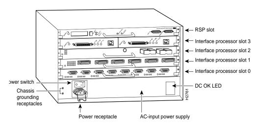
The interface processor end of the chassis also contains the AC power receptacle (a DC-input power supply is also available, but not shown), the system power on/off switch, and the DC OK power status LED, all of which are part of the power supply but accessible through cutouts in the chassis frame. (See Figure 1 or Figure 2.) To the left of the power switch and receptacle cutout is the chassis ground screw that provides a chassis ground connection for ESD equipment or a grounding wire.
